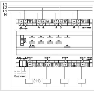
Figure 4: Device connection multi-phase
