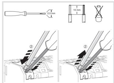
Fig 2: Installation/removal with plug-in terminals
