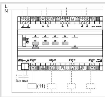
Figure 3 : Device connection 1-phase
