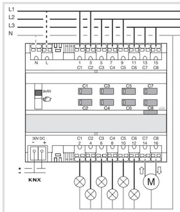
Fig 2: Device connection
