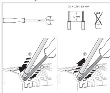
Fig 3: installation/deinstallation with plug-in terminals
