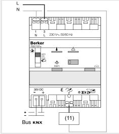
Fig 3: Device connection
