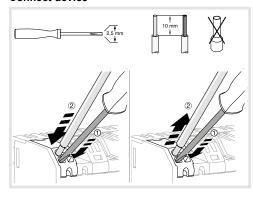
Fig 2: Installation/deinstallation with plug-in terminals
