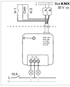
Figure 3: connection of switching loads
