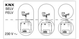
Figure 2: installation with separate terminal compartment
