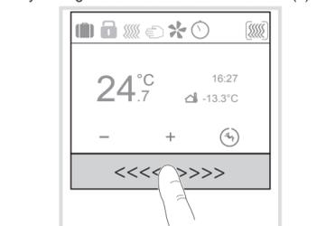
Figure 4: Slider function
