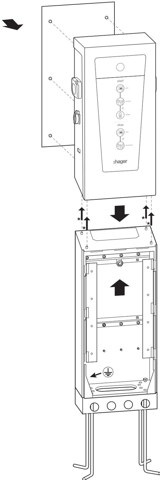
**!** The station **MUST** be mounted on its base **BEFORE** attaching the vector cabinet. The equipotential bonding must be established between the terminal, foot and base.
