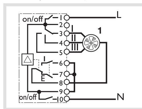
Operation of the fan (1) at the preset speed depending on the temperature. Jumper JP1 has to be off (jumper CV3-CV4 should be in the position indicated in the drawing with "CV4 ON").
