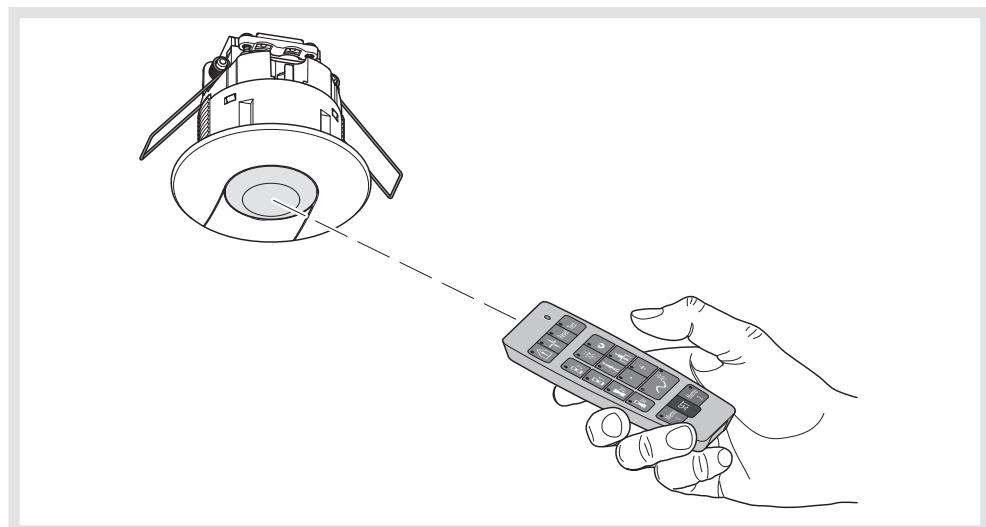
The remote control allows the user to set or modify settings on the presence detectors EE815, EE816, TCC52.E. when the potentiometer is on "auto test". It allows single and multiple settings.
