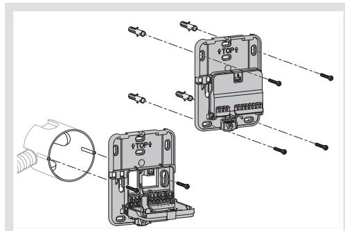
For optimum quality temperature regulation, seal the flush-mounted casing or the electrical duct.
