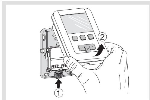
2. Open the flap with the help of a screwdriver and attach the wall-mounted base using the screws.
