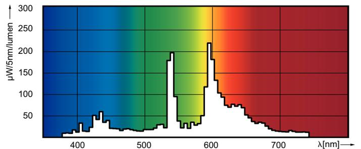
Light Distribution Diagram - MC CDM-Tm Elite Mini 20W/830 GU6.5 1CT
