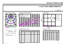
Light Distribution Diagram - CorePro LED PLT HF 18.5W 840 4P GX24q-4
