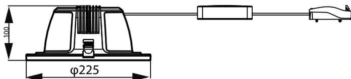
Cut-out hole diameter - Ø200mm
