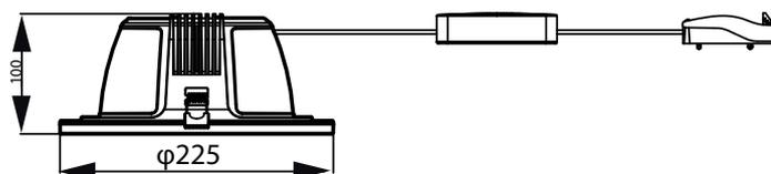
Cut-out hole diameter - Ø200mm
