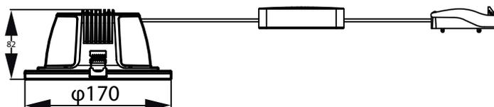
Cut-out hole diameter - Ø150mm
