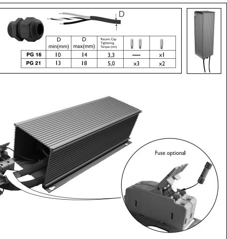
Max lamp wire cross section 4 mm<sup>2</sup>
