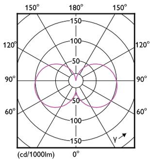
Light Distribution Diagram - CorePro R7S 118mm 7.2-60W 830
