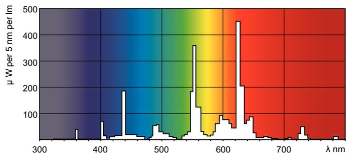
LDPB\_TL8MINI\_830-Spectral power distribution B/W
