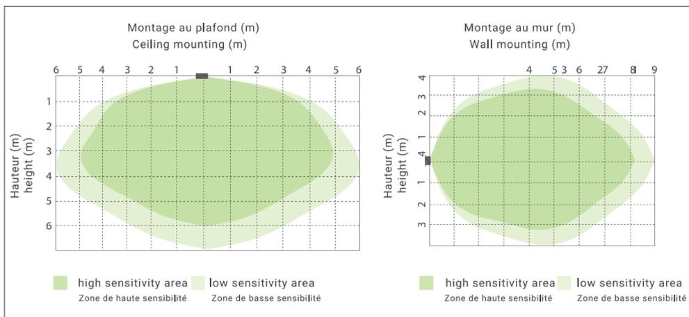
FONCTION ET CARACTÉRISTIQUE DU CAPTEUR / SENSOR FUNCTION AND FEATURE
