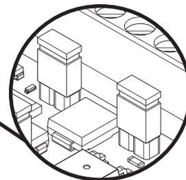
Bornier de raccordement à vis - Connection screw terminal
