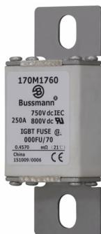
**Cartouche fusible, grande vitesse, 250 A, DC 750 V, 50 kA, size 000, 24 x 36 x 96 mm, aR, IEC, UL**
