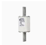
**Cartouche fusible, grande vitesse, 315 A, AC 1250 V, 100 kA, compact size 1, 45 x 45 x 156 mm, aR, IEC, UL**
