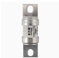
**Cartouche fusible, grande vitesse, 175 A, AC 500 V, DC 500 V, 200 kA, 29 x 92 mm, aR, UL, with indicator**
