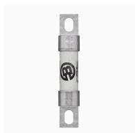
**Cartouche fusible, grande vitesse, 50 A, AC 700 V, DC 700 V, 200 kA, 21 x 112 mm, aR, UL, with indicator**
