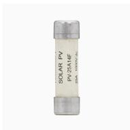
**Cartouche fusible, grande vitesse, 25 A, DC 1000 V, 30 kA, IEC 60269-6 type A, 14 x 51 mm, gPV, IEC**
