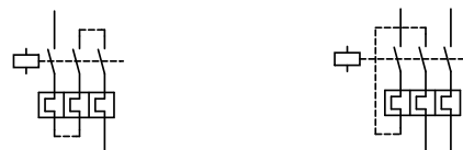
Figure 4: Wiring of the motor-protective circuit-breaker for the protection of AC or DC motors (bimetallic release switched in series)
