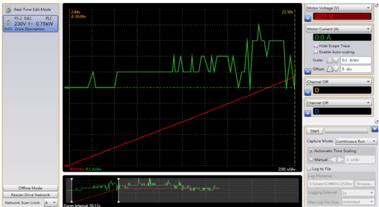
Figure 120: Moving the origin for the current signal
