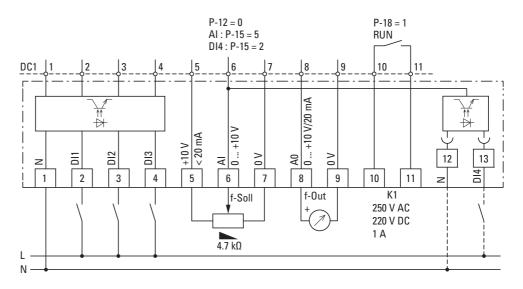
Figure 91: Block diagram DXC-EXT-IO110 and DXC-EXT-IO230
