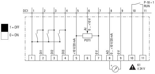
Figure 97: Block diagram DXC-EXT-LOCSIM simulator
