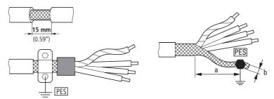
Figure 47: Screened connection cable in motor circuit
