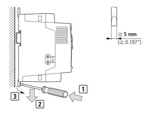
Figure 30: Dismantling from mounting rails
