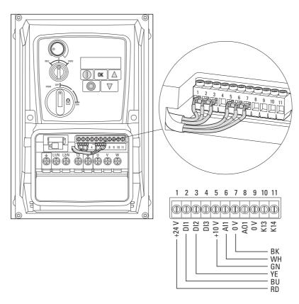
Figure 61: DC1-...A6S... (connection wired at the factory)
