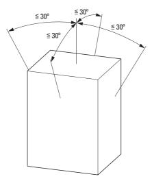
Figure 23: Mounting position
