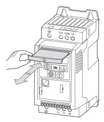
Figure 75:Help cards in units with an IP20
