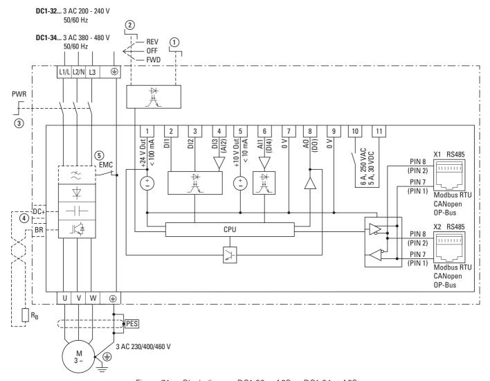
Figure 71: Block diagram DC1-32...-A6S..., DC1-34...-A6S...
