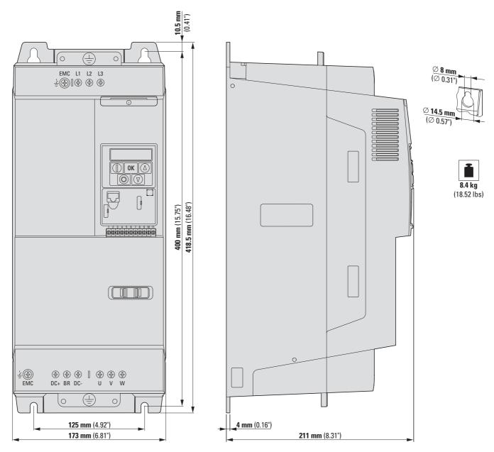
Figure 80: Dimensions and weight for DC1 with frame size of FS4 and IP20 (NEMA 0) degree of protection
