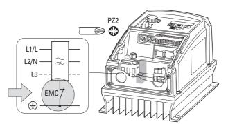
Figure 38: EMC screw in protection class IP66
