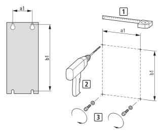
Figure 27: Mounting dimensions
