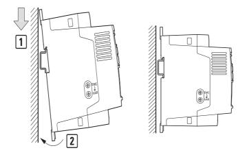
Figure 29: Fixing on a mounting rail
