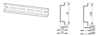
Figure 28: Mounting rail conforming with IEC/EN 60715
