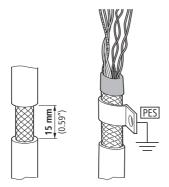
Figure 54: Screen termination at one end (PES) close to the variable frequency drive
