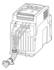
Figure 46: Connection on motor side
