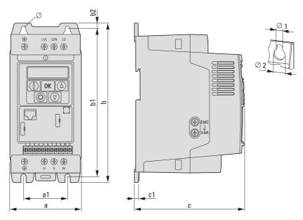
Figure 79: Dimensions for DC1 with IP20 degree of protection (NEMA 0)
