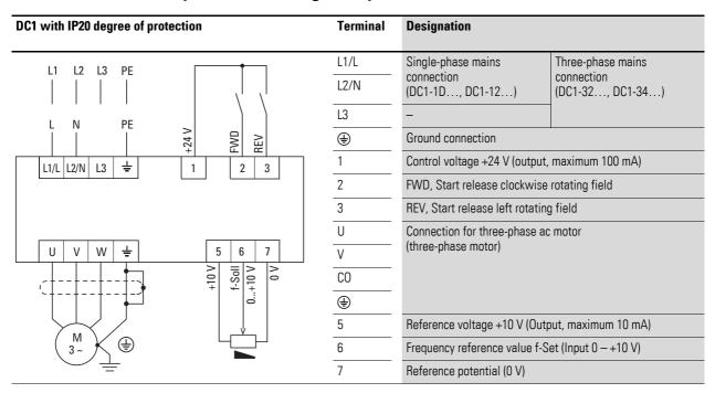
The potentiometer should have a fixed resistance (connection to control terminals 5 and 7) of at least 1 k $\Omega$  and up to a maximum of 10 k $\Omega$ . A standard fixed resistance of 4.7 k $\Omega$  is recommended.
