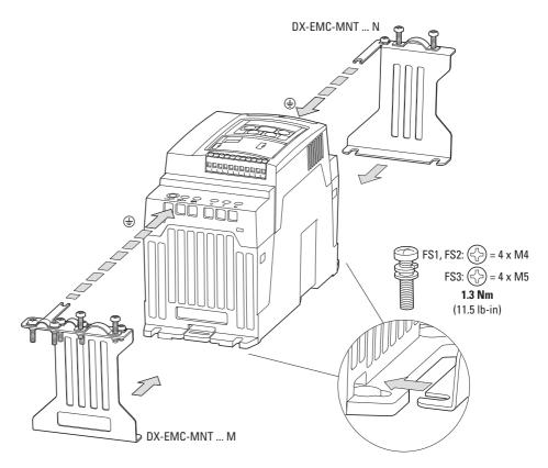
Figure 40: EMC cable brackets (example: FS2 frame size)
