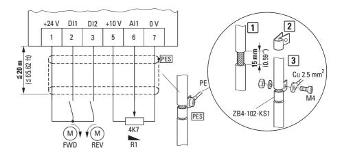
Figure 53: Simple connection example
