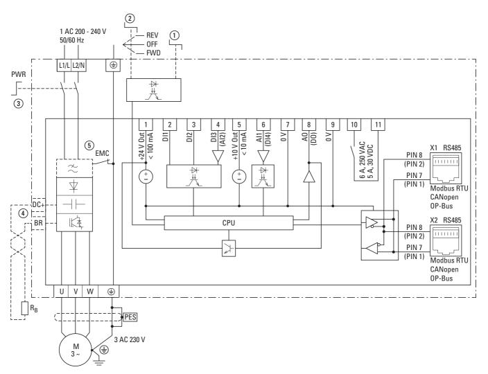
Figure 69: Block diagram DC1-12...-A6S...
