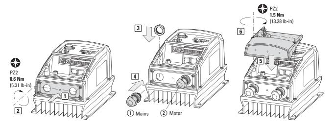
Figure 50: Installaling the cable glands
