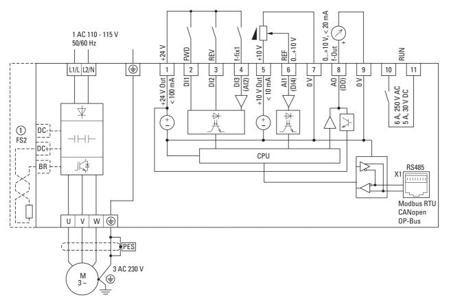
Figure 63: Block diagram DC1-1D...Nx-...
