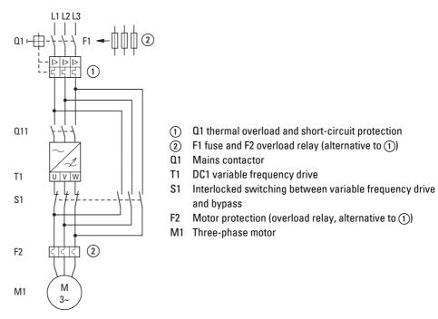
Figure 18: Bypass motor control (example)
