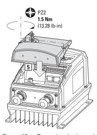
Figure 43: Removing the lower housing cover
