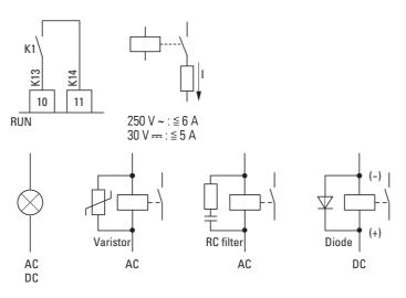
Figure 58: Connection examples with suppressor circuit
