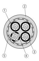
Figure 48: Four-core, screened motor supply cable
