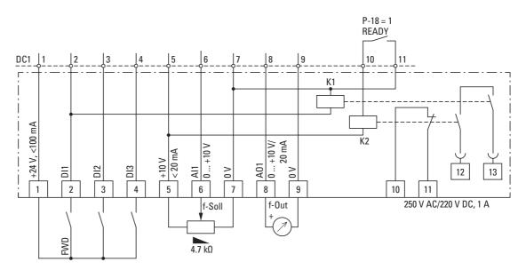
Figure 95: Block diagram DXC-EXT-2RO1AO
