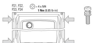
Figure 32: Openings for fixing screws
