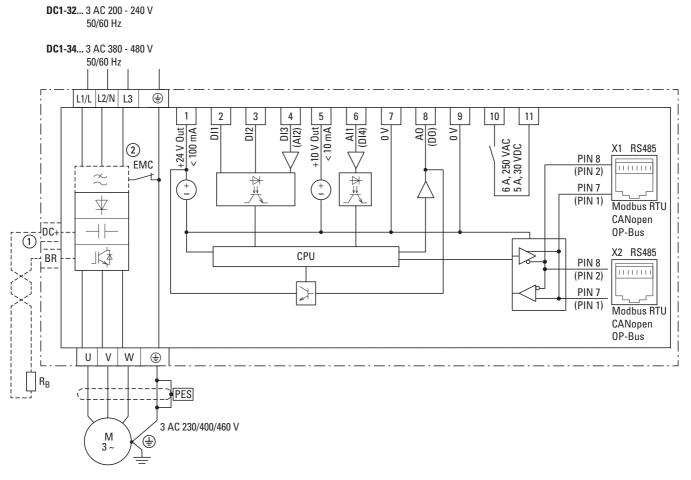
Figure 72: Block diagram DC1-32...-A66..., DC1-34...-A66...
