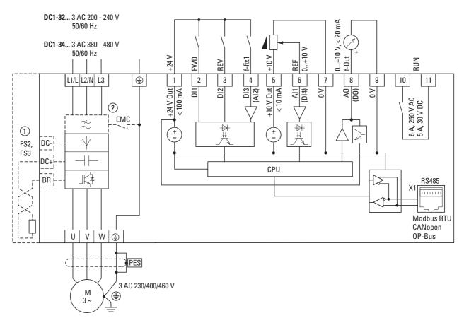
Figure 65: Block diagram DC1-32... and DC1-34... in frame sizes FS1, FS2 and FS3
