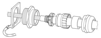
Figure 51: Example: diagram of EMC gland assembly
