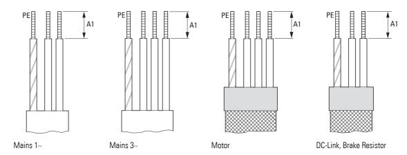
Figure 44: Stripping lengths in the power section
