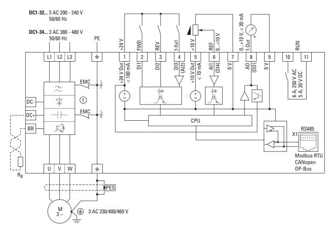
Figure 66: Block diagram DC1-32... and DC1-34... in frame size FS4
