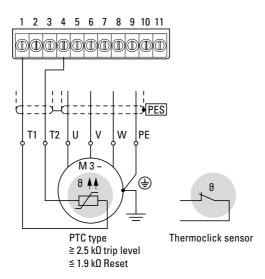
Figure 62: Thermistor connection
