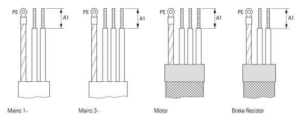
Figure 45: Stripping lengths in the power section
