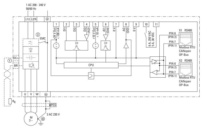
Figure 70: Block diagram DC1-12...-A66...
