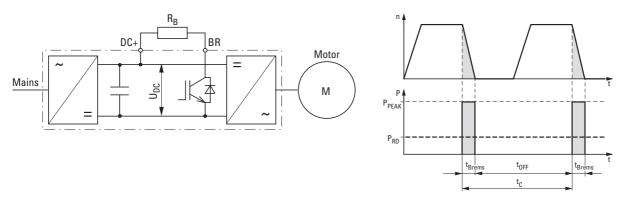
Figure 16: Braking cycle, fast motor stop with external brake resistor
