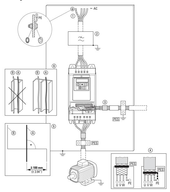
Figure 41: EMC installation
