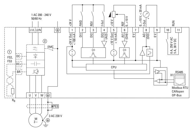
Figure 64: Block diagram DC1-12...
