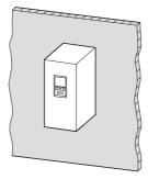
Figure 22: Surface mounting on metal plate
