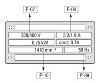
Figure 78: Motor rating plate, P-08 = 1.9 A at 400 V
