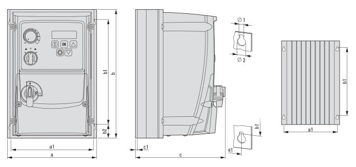
Figure 81: Dimensions for DC1 with IP66 degree of protection (NEMA 4X)
