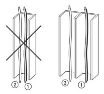
Figure 35: Separate routing
