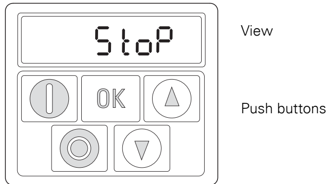
Figure 1: Operating unit view
