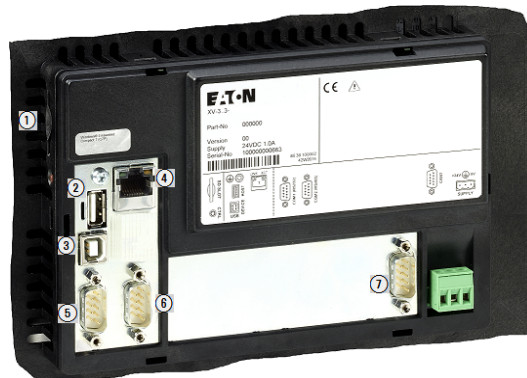
Figure 28: Interfaces included on all HMI panels
