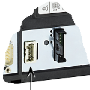
Figure 36: SmartWire-DT power connector
