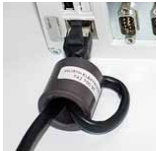
Fig.. 43 Ethernet cable, double loop through ferrite
