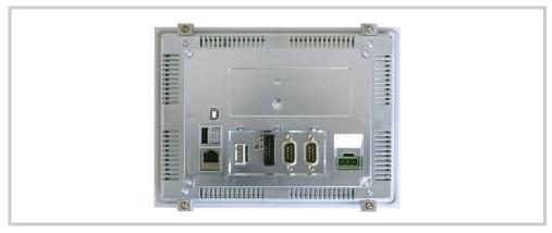
Abb. 28 Devices with four retaining brackets (do not meet IP65 / NEMA 4X requirements)
