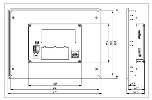
Abb. 32 Mechanical dimensions of the 8.4" devices in mm
