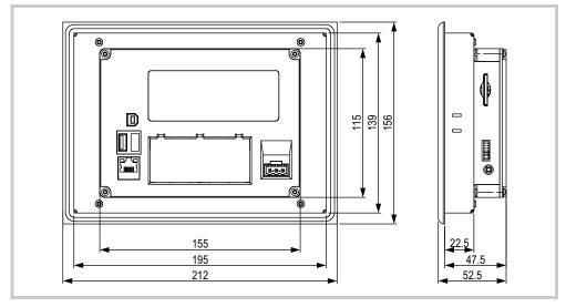
Abb. 31 Mechanical dimensions of the 5.7" devices in mm
