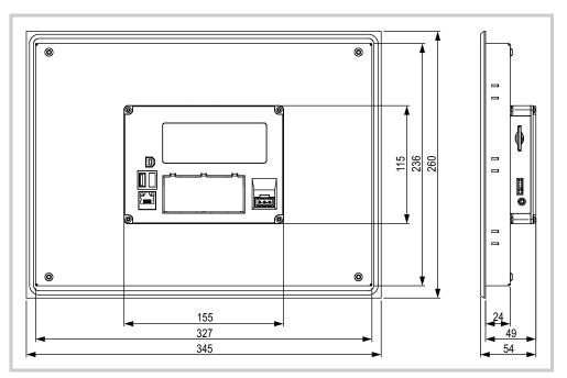
Abb. 33 Mechanical dimensions of the 10.4" devices in mm
