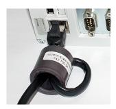
Abb. 34 Ethernet cable with double loop through ferrite core
