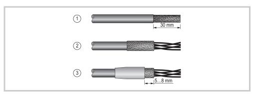
Abb. 5 Connecting the cable shield
