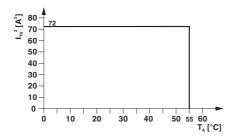
Figure 3: Derating curve
