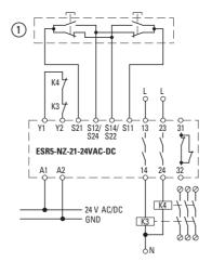
Figure 4: Two-hand control device
