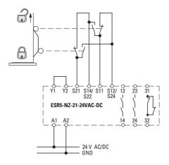
Figure 5: Guard - two-channel
