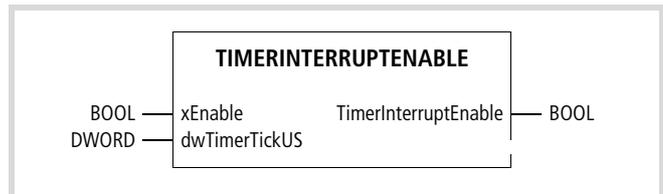
Figure 49: TimerInterruptEnable function
