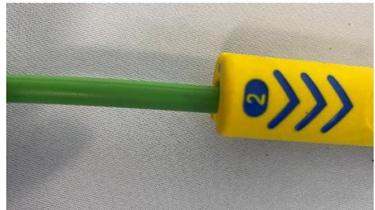
4. Make a 45° radial cut to the right on the sheath and return to 0
