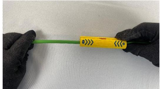
3. Press the cutting tool to close it and make a cut on the sheath
