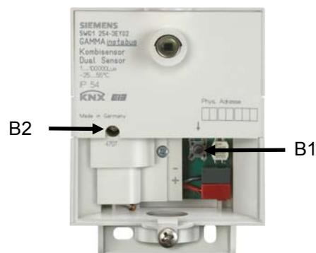
Figure 2: Location of display and operator elements
