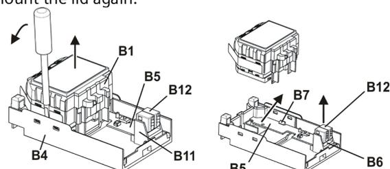
figure 6: dismounting an RS module
