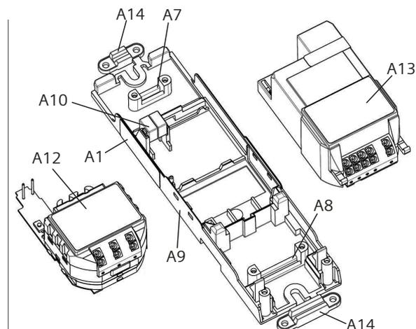
figure 4: mounting / dismounting of RS/RL modules
