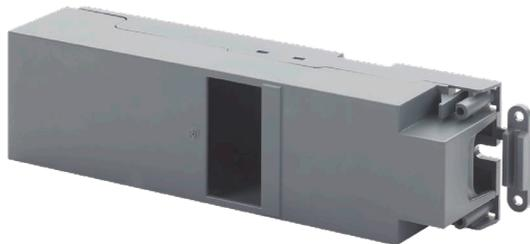
The AP 118 Control Module Box with a height of 41 mm is designed for installation in a false ceiling, in a raised floor, directly on a wall or in an installation channel or raceway. The Control Module Box is affixed with screws at the two ends of the housing.
