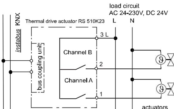
figure 1: Example of operation
