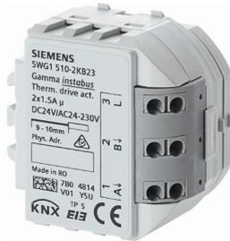
The RS 510K23 Thermal drive actuator is a KNX device with two switching outputs (2 x 1.5A) for control of thermal drive actuators. The device is installed in an AP 118 Control Module Box or an AP 641 Room Control Box. The bus is connected via a bus terminal block. The device electronics are supplied via the bus voltage.
