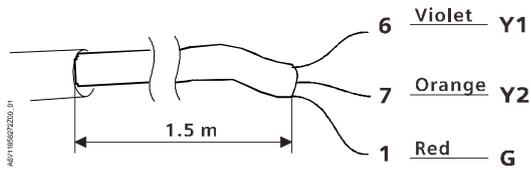
Y1 = signal de commande OUVERTURE (24 V~)
