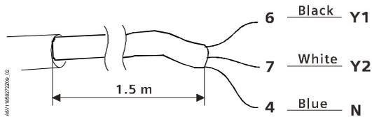
Y1 = signal de commande OUVERTURE (230 V~)
