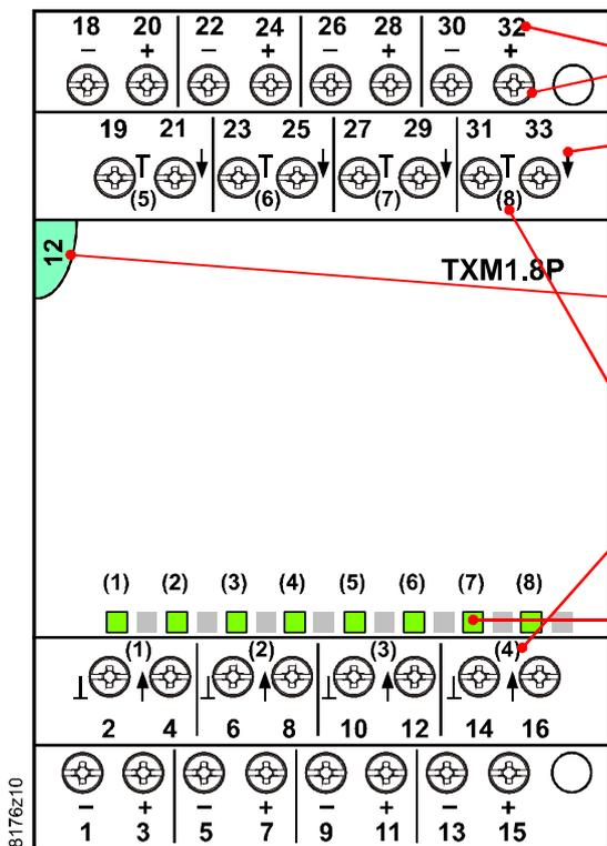
Connection terminals (No. 1 screwdriver for slotted or recessed-head \* screws) with test plug socket (pins 1.8...2 mm) and terminal number.
