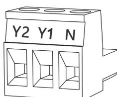
Y2 = signal de commande FERMER (230 V)
