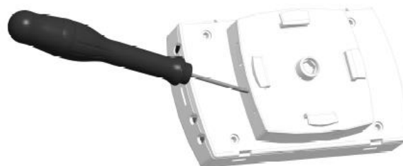
Fig. 2: Position the screwdriver to break out the security windows
