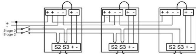
Fig 6a. BExCS110-05D AC Simplified Block Diagram for simultaneous operation (positive switching)
