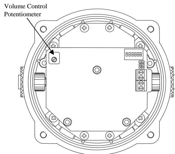
Fig. 9 Location of Volume Control Potentiometer
