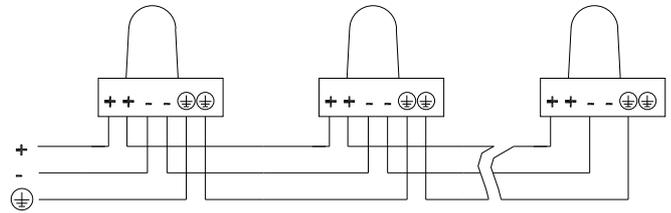
Fig. 5. E2xB05/E2xB10 DC Simplified Block Diagram
