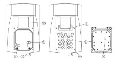
Plug the ribbon cable onto the pin contact strip (7) of the keypad plate. Tighten the keypad plate (6) using four screws (8).
