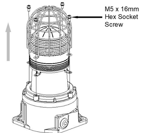
Figure 7: Removal of Lens.
