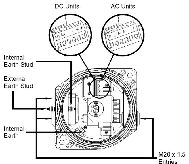
Figure 5: GNEXB2 Entries and Terminal Blocks.
