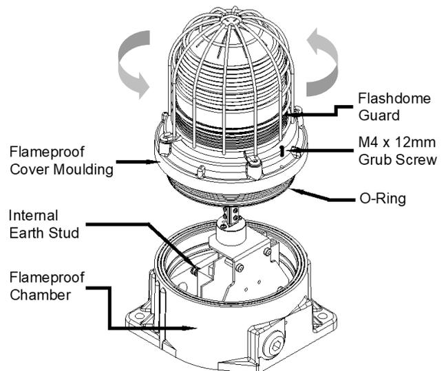
Figure 3: Accessing the Explosion Proof Enclosure.
