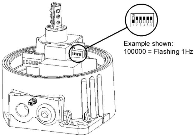
Figure 6: DIP Switch Location.
