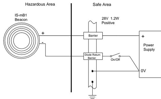
Fig 4 Single stage alarm using two channel barrier.
