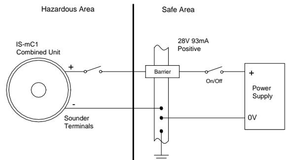
Fig 4 Sounder single stage alarm using single channel barrier.
