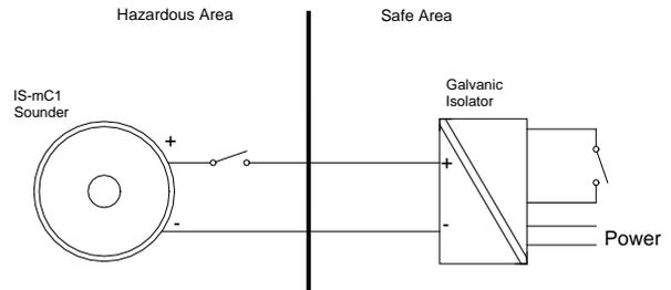
Fig 9 Sounder single stage alarm using galvanic isolator.
