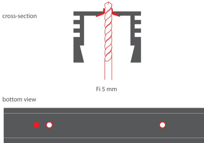
**2.** Mount the fasteners to the extrusion. Manual for the DP fastener can be downloaded from [www.klusdesign.eu](http://www.klusdesign.eu).
