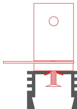
**3.** Mount the LED strip in the extrusion and lead the cables through pre-drilled holes. Then lead them to the connector of the DP-ZZ fasteners. Each hole should lead a cable with one power pole, LED strip has to be cut before installation, so the wires can be easily routed to the holes.
