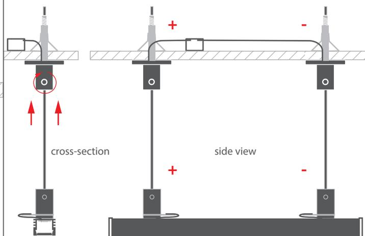
**1.** Drill a holes with a diameter of 5 mm in the selected extrusion. 3 holes are needed to mount the fasteners and lead powering cable. Bevel the 2 holes for the fasteners so that the plastic screw head fits in.
