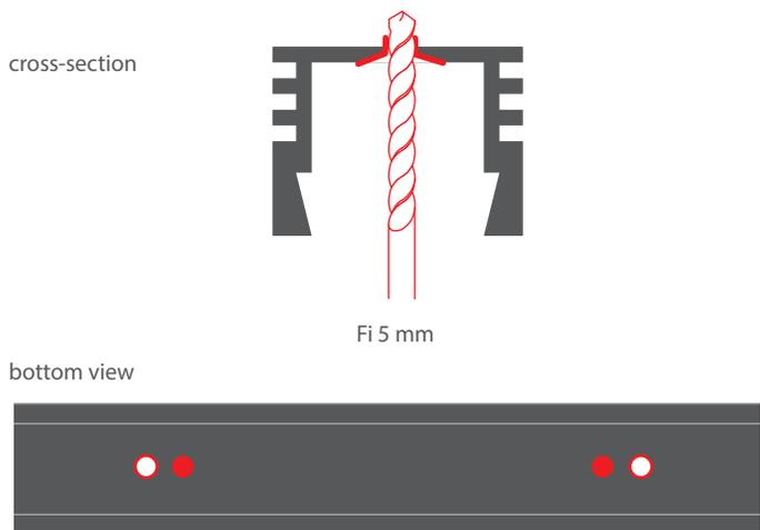
**2.** Mount the plastic screw in the beveled holes, on the top mount the assembled plastic base, small power connector and head. Manual for the DP-ZZ fastener can be downloaded from [www.klusdesign.eu](http://www.klusdesign.eu).
