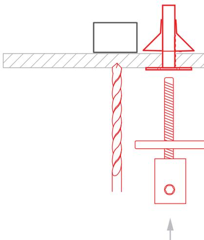
**6.** Mount the fixture with rods into the ceiling fasteners. Connect the cable to the power supplier, leading it through a pre-drilled hole in the ceiling.
