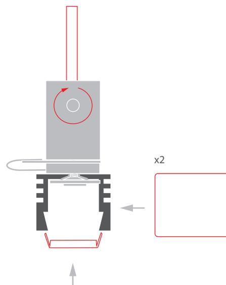
**5.** Install the W-KG-Z ceiling fasteners. The fastener installation manual can be downloaded at [www.klusdesign.eu](http://www.klusdesign.eu). Connect the cables, each for the single power pole to the fasteners. The cables should go through a pre-drilled hole just under the masking cover of the fastener.
