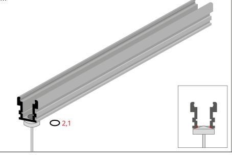
Chamfer the hole to hide the hermetic coupler item (2.1) in the recess.
