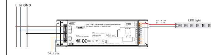
Modify the DALI address when the product is controlled by a DALI bus:
