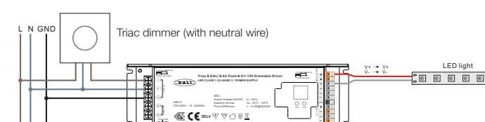
If multiple power supplies are controlled in parallel, be sure to set the minimum dimming level on the controller to prevent flickering.
